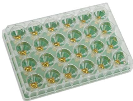
Our standard 24-well plates feature 12 electrodes per well with an opaque epoxy substrate base. This version is also available with a transparent glass base with PEDOT-coated gold electrodes.
